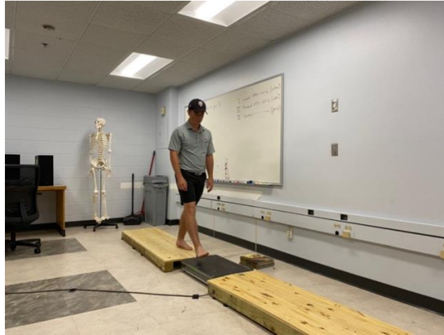
Figure 3. Recording of ground reaction forces. The participant walks at a self-selected speed on the force plate.
